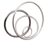
Hollow metal O-ring is made by heat resistant and noncorrosive stainless steel pipe. It is available to have small holes in the inner diameter or outer diameter, when the pressure increasing, the self-sealing function will be work. The hollow O-ring with small holes is specially applied when the pressure over than 70kgf/cm², the pressure resistant will better than no holes O-ring. Upon customer's requirement, we also offer O-ring surface coating PTFE or silver.
